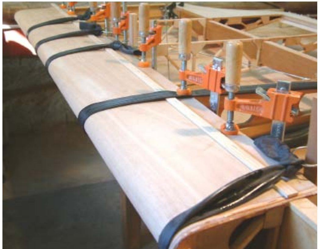
The leading edge (1 mm ply) was attached in two lengths, secured with innertube clamps.
