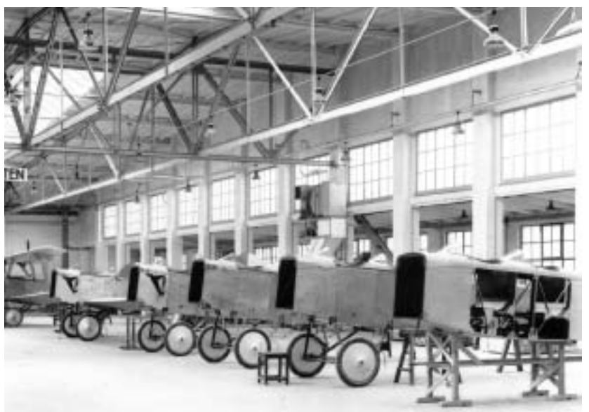
Udet U-12 Flamingos in production. The Flitzer owes a lot to its design.
