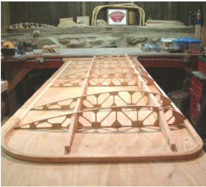
Flashback: First trial fit of the wing parts on January 1.
