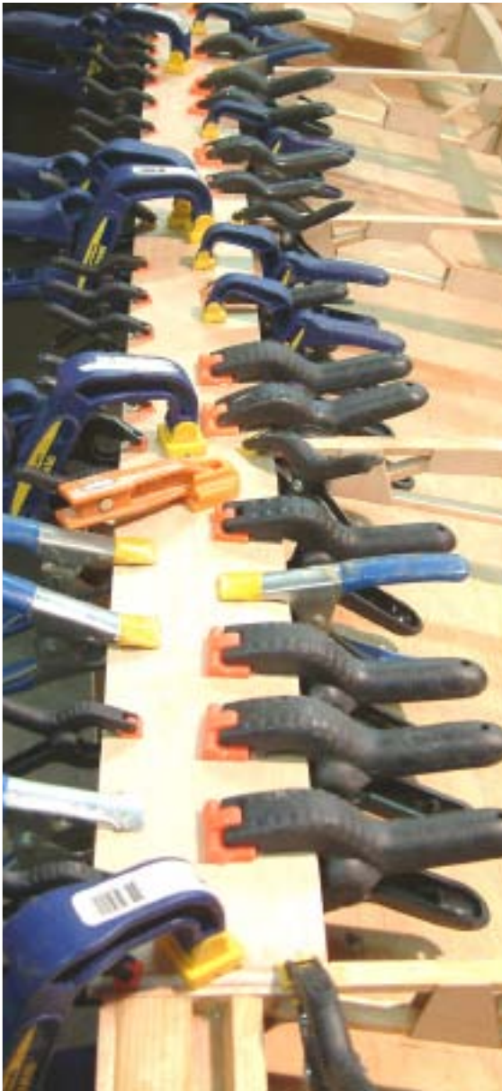
Trailing edge plywood is clamped gently in place.
