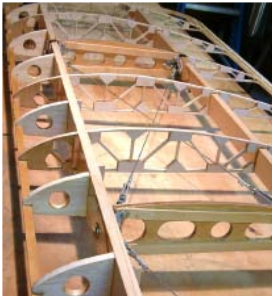
Wing structure takes shape, bracing wires fitted.
