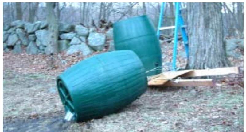
Twang!!! The aircraft wire held, but a steel hook on the test rig failed.
