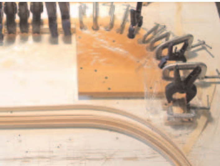
Wingtip laminations were bent wet in this jig, allowed to dry, then glued.
