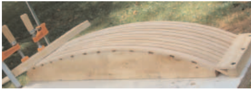
Capstrips for all the wing ribs were steamed and then bent in this simple jig.
