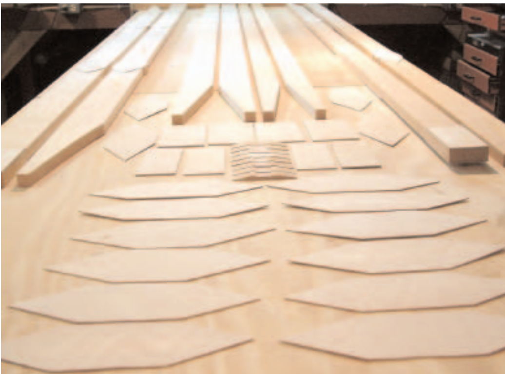
The spars and their plywood reinforcing plates that spread stress all around. A lesson there for all of us!
