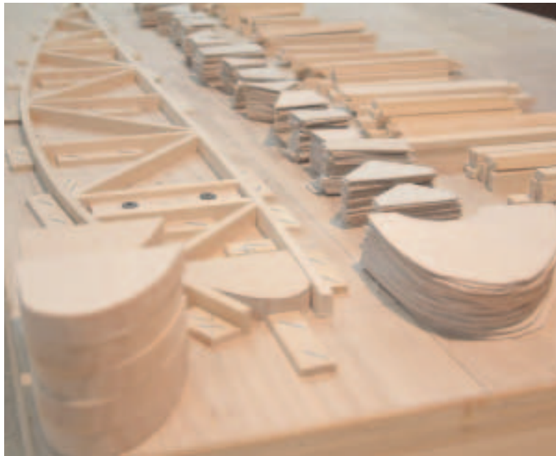
Wing ribs were glued, stapled in the jig, taken out and the other side done straight away.
