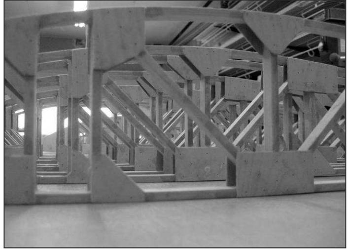
THE UPPER AND LOWER WING RIBS ARE ALMOST COMPLETED. ONLY NEED TO FORM RIB NOSE AND CUT THE END. THE LOWER OUTER RIBS WERE SIMPLIFIED MORE LIKE THE UPPER RIBS.
