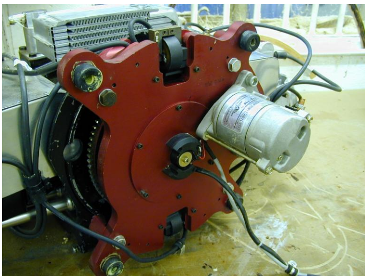
BACKPLATE REVERSED TO PLATE STARTER MOTOR ON R.H. SIDE
