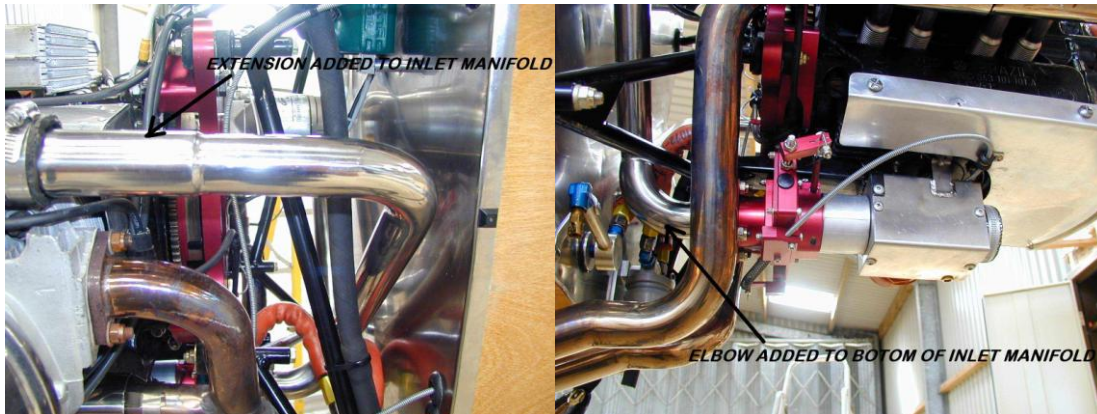
EXTENSION TO INLET MANIFOLD 90° BEND ADDED TO INLET MANIFOLD
